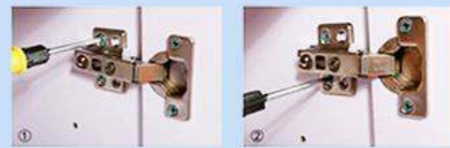
Door panels are uneven
